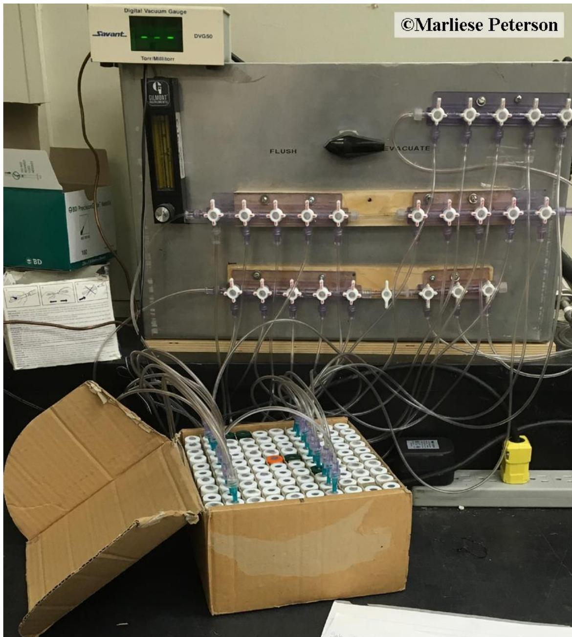
Figure I. Evacuation apparatus / manifold (Note the valve is currently set to “Flush”)
