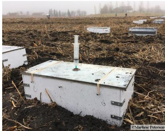
Figure 3. A sealed rectangular static vented chamber
