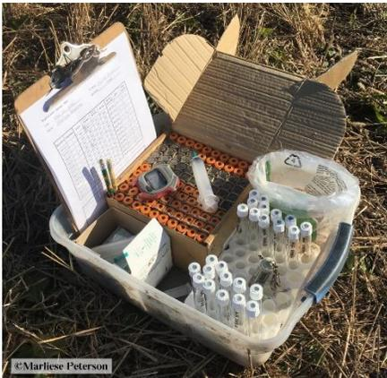
Figure 2. A fully stocked gas sampling kit
