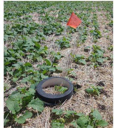
Figure 4. A round static vented chamber/collar
