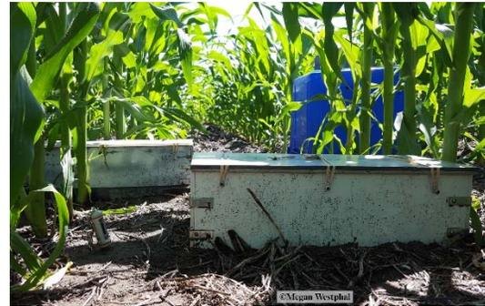
Static-vented chambers (white) for monitoring  $N_2O$  flux
