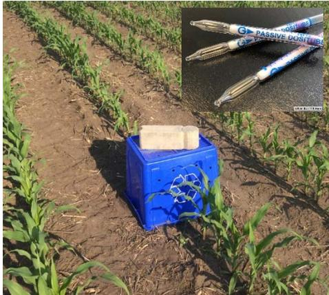
Custom-made chamber and passive colorimetric dosimeter tubes for measuring NH<sub>3</sub> emissions
