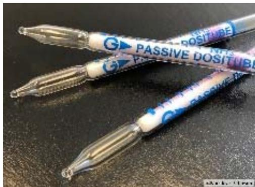
Passive colorimetric dosimeter tubes for measuring NH<sub>3</sub> emissions
