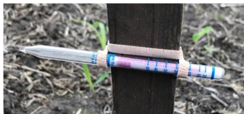
Figure 3. Left: a field technician installing an ammonia dositube stake; Middle: an active ammonia dositube mounted to a stake; Right: an ammonia dositube chamber held in place with a patio brick
