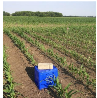
Figure 3. Left: a field technician installing an ammonia dositube stake; Middle: an active ammonia dositube mounted to a stake; Right: an ammonia dositube chamber held in place with a patio brick
